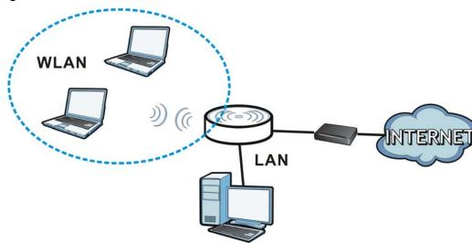
Figure 14 Wireless Internet Access in Access Point Mode
