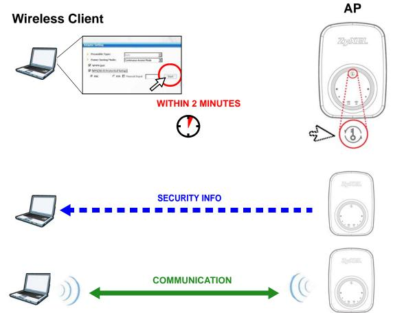
Figure 18 Example WPS Process: PBC Method
