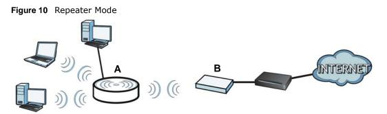
After the WRE6505 v2 and the access point connect, the WRE6505 v2 acquires its IP address from the access point. The clients of the WRE6505 v2 can now surf the Internet.
